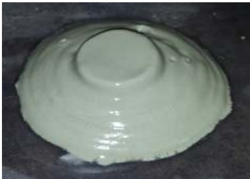
Fig. 2. Form of paste after lifting cylinder
