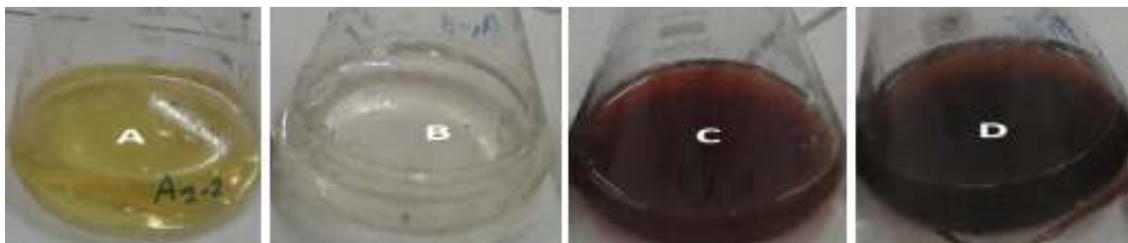
Fig. 3. Silver nanoparticles biosynthesis by A. terreus A2-2. (A) Biomass filtrate of A. terreus A2-2 without \text{AgNO}_3 (pale yellow color); (B) Only \text{AgNO}_3 solution (colorless); (C and D) biomass filtrate of A. terreus A2-2 reacted with aqueous solution of 1.5 mM \text{AgNO}_3 ; the color is gradually changed from pale yellow to brown after 24 h at 35°C and pH 10
