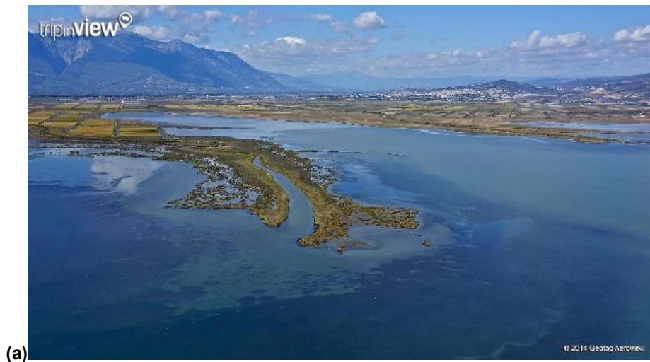
Fig. 10. Along the coastal zone, of Iria (eastern coast of the Argolic Gulf) and the small town of Tolo, shoreline erosion processes have occurred. Human intervention is very important and includes the construction of a fishery shelter, a road parallel to the shoreline and in a small distance from it, regulation torrent's channels and the arbitrary installment of small groins. All the aforementioned interventions seem to have either initiate and/or enhanced erosion, which locally accounts several meters, despite the non-intense nearshore hydrodynamic conditions. Coastal erosion and shoreline retreat are expected to be increased due to Climate Change and the potential future Sea-level rise (Photos by Mertzani As.-July 2019)
