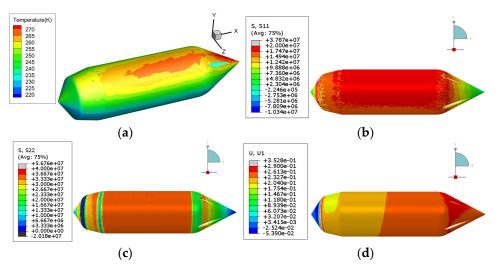
**Figure 8.** Simulation results at 12:00 p.m. (**a**) Temperature distribution at 12:00 p.m. (**b**) S11 stresses at 12:00 p.m. (units: Pa) (**c**) S22 stresses at 12:00 p.m. (units: Pa) (**d**) U1 deformation at 12:00 p.m. (units: m).
