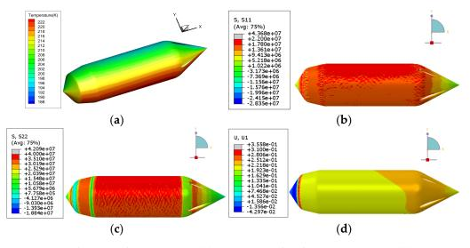
Figure 10. Simulation results at 12:00 a.m. (a) Temperature distribution at 12:00 a.m. (b) S11 stresses at 12:00 a.m. (units: Pa) (c) S22 stresses at 12:00 a.m. (units: Pa) (d) U1 deformation at 12:00 a.m. (units: m).
