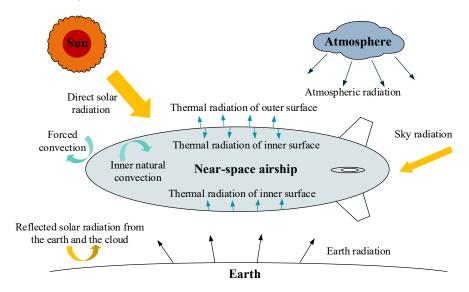
Figure 2. Near-space airship thermal environment.
