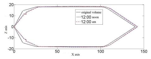
Figure 13. The comparison of airship shapes (X-Z view) (units: m).
