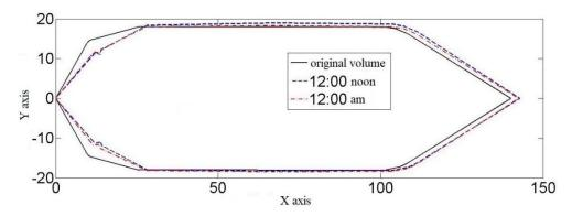
Figure 12. The comparison of airship shapes (X-Y view) (units: m).
