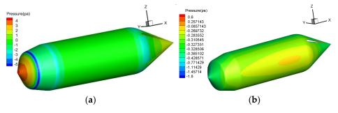
Figure 6. Static pressure of the envelope. (a) Forced convection pressure. (b) Natural convection pressure.
