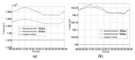
Figure 11. Changes in airship volume and length. (a) Airship volume. (b) Airship length.
