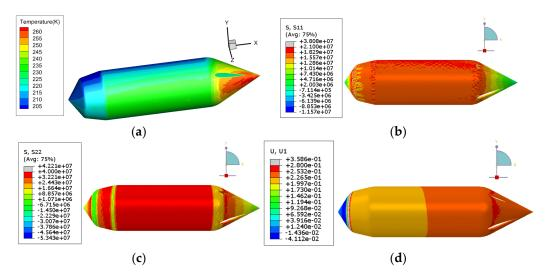
**Figure 9.** Simulation results at 6:00 p.m. (**a**) Temperature distribution at 6:00 p.m. (**b**) S11 stresses at 6:00 p.m. (units: Pa) (**c**) S22 stresses at 6:00 p.m. (units: Pa) (**d**) U1 deformation at 6:00 p.m. (units: m).
