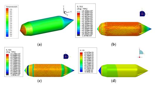
**Figure 7.** Simulation results at 6:00 a.m. (**a**) Temperature distribution at 6:00 a.m. (**b**) S11 stresses at 6:00 a.m. (units: Pa) (**c**) S22 stresses at 6:00 a.m. (units: Pa) (**d**) U1 deformation at 6:00 a.m. (units: m).
