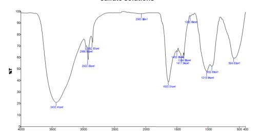
Fig. 3. FT-IR Analysis of *Tecoma stans* mediated copper oxide nanoparticles
