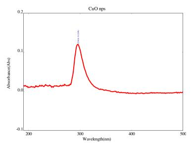
Fig. 1. UV-visible spectra of *Tecoma stans* mediated copper oxide nanoparticles
