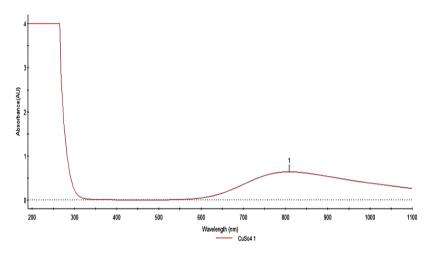
Fig. 2. UV-visible spectra of the reaction mixture of leaf extract of Tecoma stans with copper sulfate solutions
