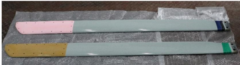
**Figure 2.** Test blades coated with PSP and TSP.
