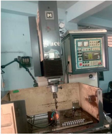
FIGURE 2: Machining process of PMEDM.
