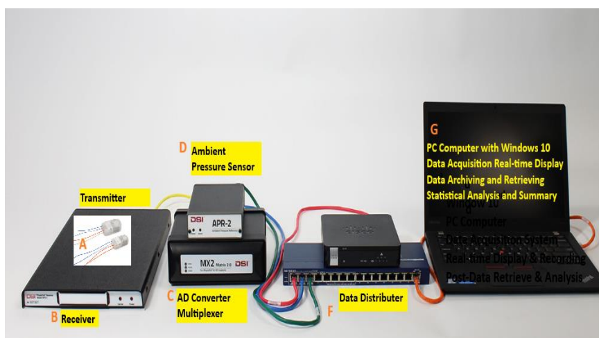
Fig. 2. Our telemetric data acquisition system, which consists of a transmitter, receiver, AD converter, and multiplexer
