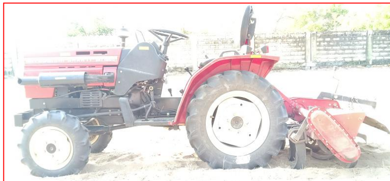
Fig. 2. Developed active - passive combination tillage implement with test tractor
