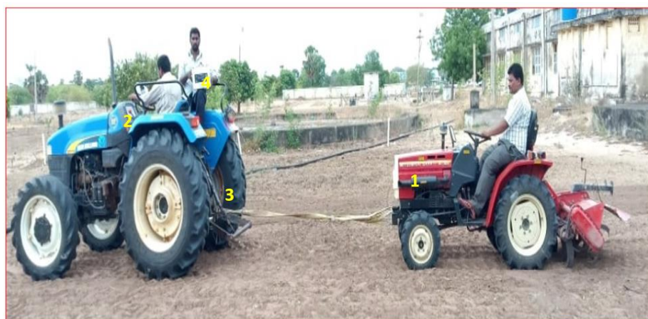
Fig. 6. 1. Implement with test tractor; 2. Auxiliary tractor; 3. Load cell; 4. Digital dynamometer
