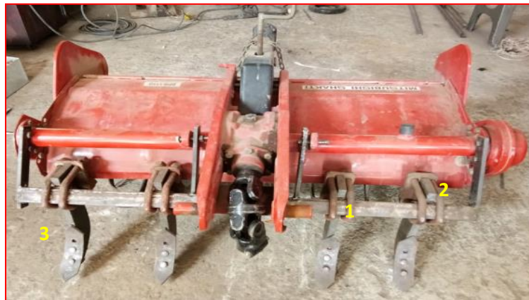
Fig. 1. Developed active - passive combination tillage implement 1. Supporting frame; 2. Supporting arms; 3. Tines
