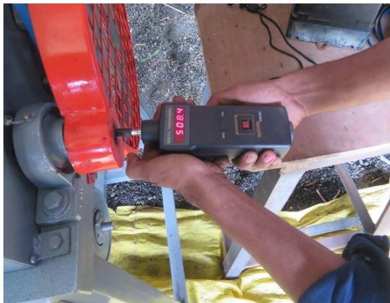
Fig. 5. Measurement of the speed of the prime mover, cylinder, and feed roller using a digital tachometer during no load and load conditions
