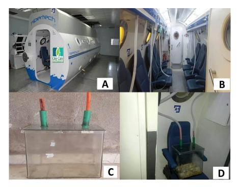
Fig. 1. The hipertech multiplace double compartment hyperbaric chamber used in AVC (A). The eight chairs room of the multiplace HBO chamber (B). The locally manufactured HBO chamber for small animals (C). The small animal chamber inside the isolated room of HBO chamber during the session (D)
