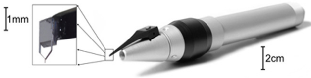
Figure 1. Illustration of the 2d-Laser Cantilever Anemometer with a detailed view of the cantilever.
