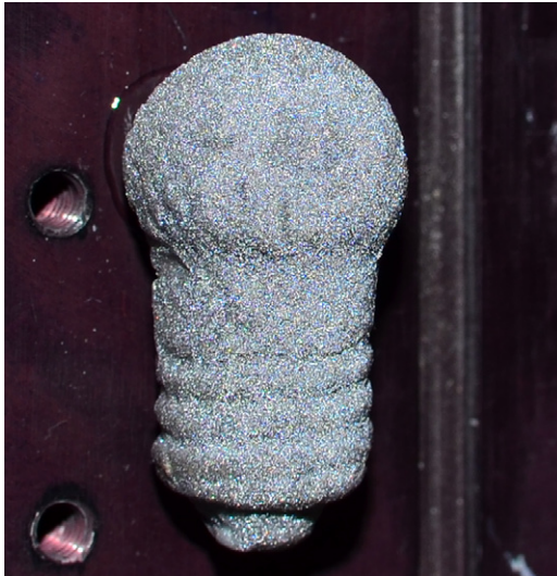
Figure 6. Light bulb coated with reflective paint that was used to demonstrate the interferometer's surface contouring ability.
