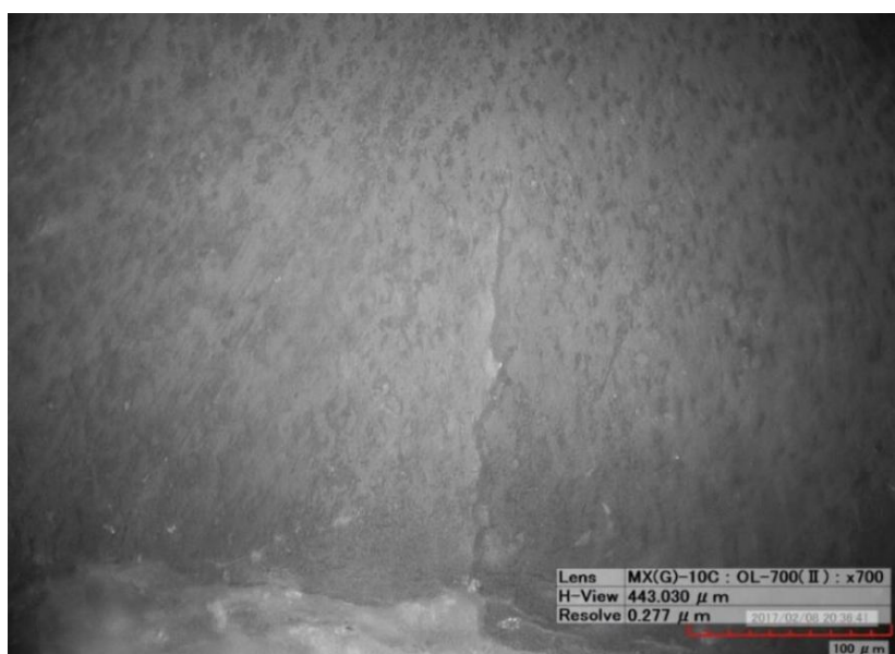
Fig. 1. A photograph of micro crack mag 700x
