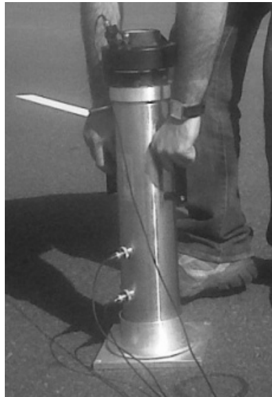
Fig. 1. Impedance Tube Placed Against the Steel Plate
