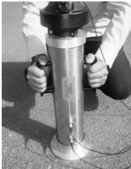
Fig. 3. In-situ measurement of road sound absorption coefficient by Impedance Tube
