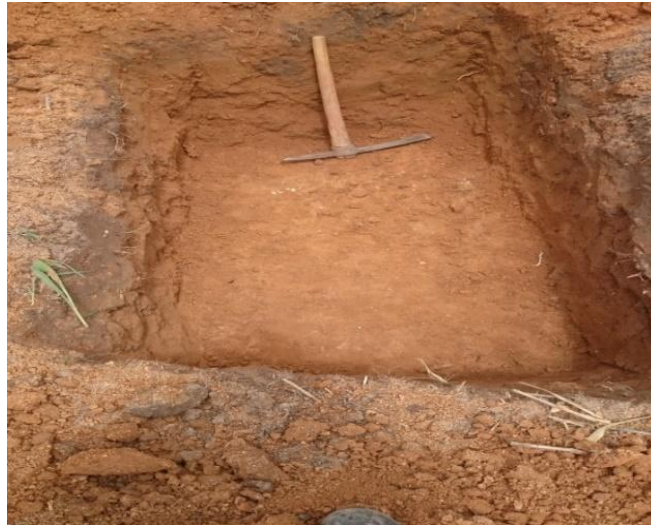
Fig. 9. Typical tests pits excavated at the site
