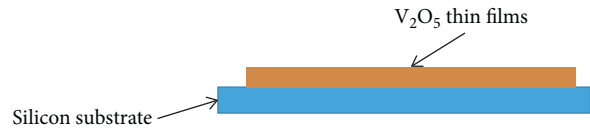
FIGURE 1: V_2O_5 thin film deposition using PLD.
