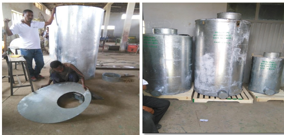
Fig. 2. Manufacturing of different sized air tight silos manufactured in MAMREREC, 2018
