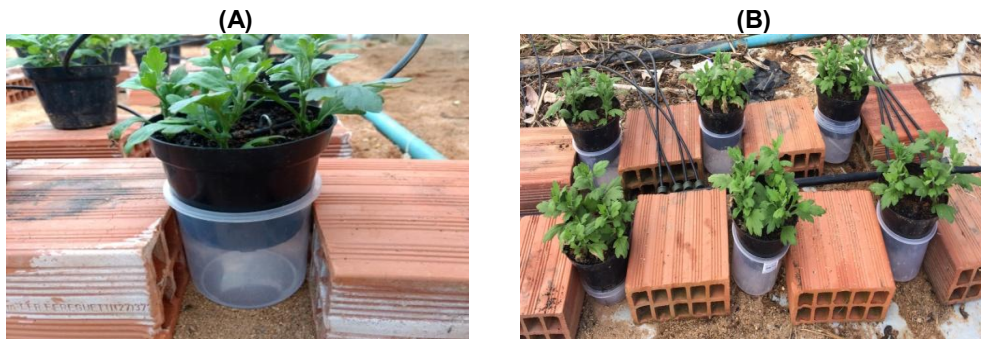
Fig. 1. Drainage lysimeter (A) and overview of the six drainage lysimeters (B)
