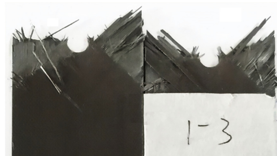
Figure 9. Photograph of failed laminate specimen.
