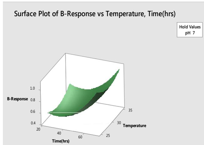
Fig. 4. Response surface plot of B-response vs. temperature, time(hrs)
