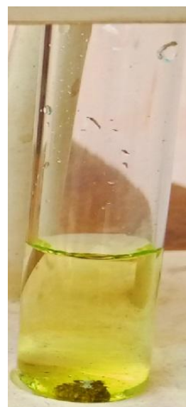
Fig. 8. Effect of selectivity on the colorimetric sensing of I^- ions by PCAFC-Cu(II)
