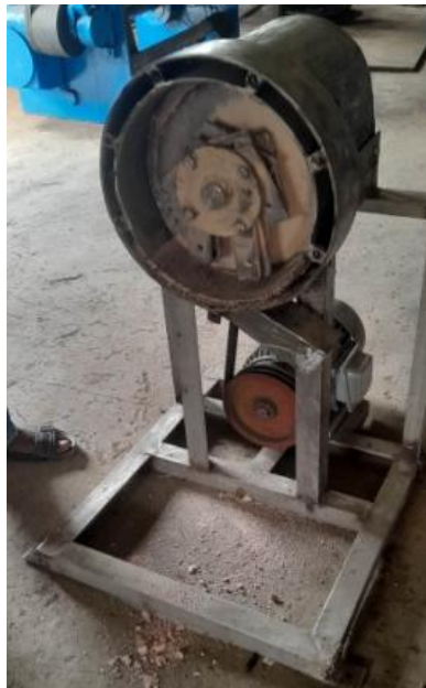
Fig. 3. Picture of the Uncoupled Hammer Mill Machine to show the grinding chamber (hammer mills and compartment)
