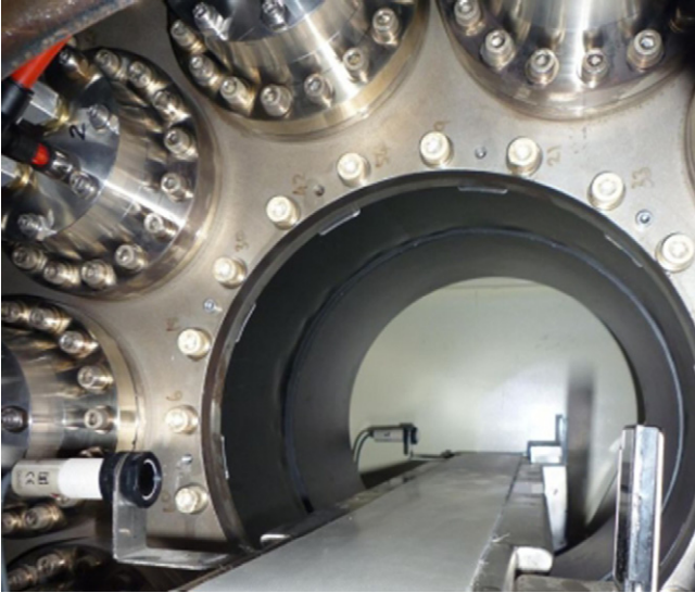
Figure 1. View of the RTT20 tunnel and conveyor belt, showing the vacuum tube and electron gun assembly.
