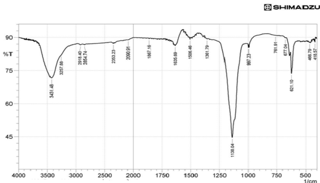
Fig. 1. FTIR spectrum of ZnS powder
