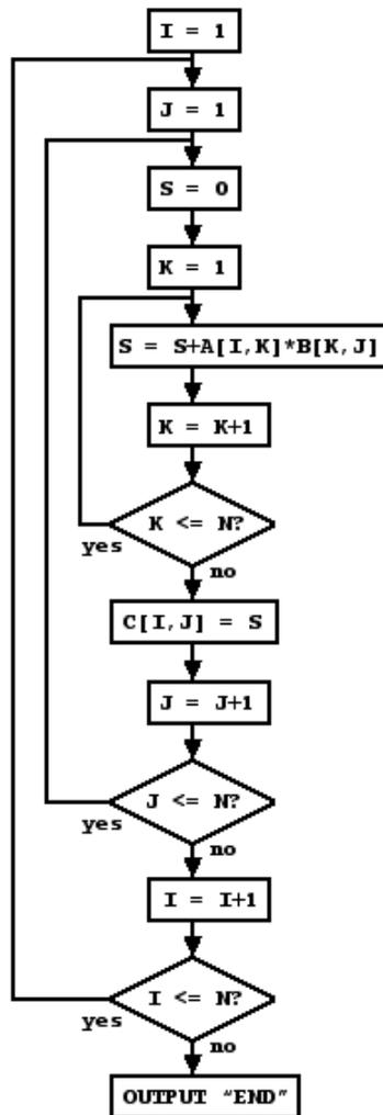
Fig. 4.1. A matrix-product program with a feedback vertex
